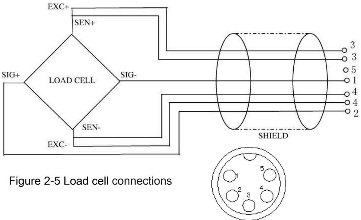
Figure 2-5 Load cell connections
