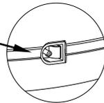
Plug the AC adaptor to the AC adaptor socket on the back. The AC input requirement could be 110,120,220,230 or 240Volts (50/60Hz) depending on the area where used, so please verify that the adaptor is correct
