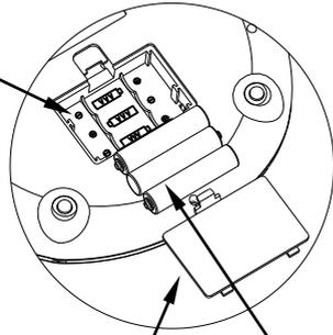
Remove the battery compartment cover and insert three batteries(AAA size) into the battery compartment, taking extreme care that the polarities plus and minus is observed.
