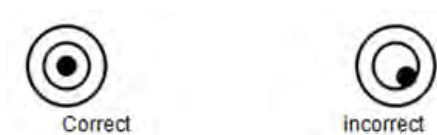
Fig. 3.2 Correct leveling with the aid of the bubble level
