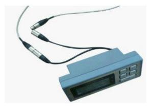
Step1: Connect the cable to the load cell and plug the metal connectors under power off condition.
